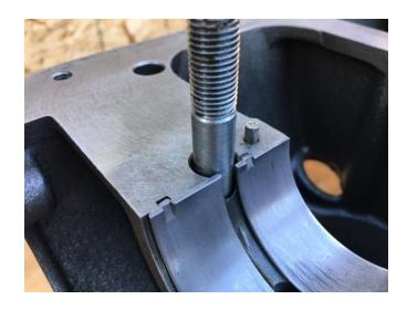
The connecting rod big end comes very close to the cylinder block walls, oil pan walls, and the camshaft. Verify that there is clearance by rotating the crankshaft after assembly of each connecting rod/piston assembly.
