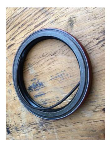
The garter spring side of the seal needs to be installed towards the interior of the engine. The seal must be needs to be driven evenly until it bottoms out. The seal cavity is deep enough for 2 seals. If 2 seals are used, leave a cavity between seals and fill the cavity with a high quality oil.
