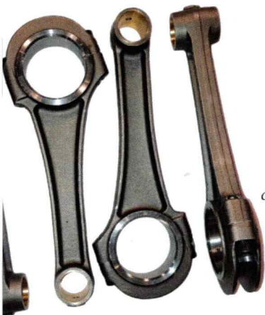
Modern insert bearings insure easy serviceability and less friction.
