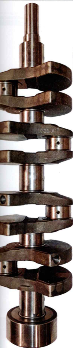
The main bearing crankshaft and block have 2" bearings at the crank journals & rods.
