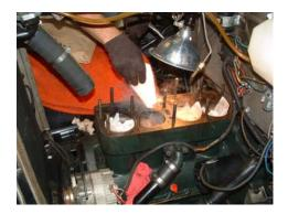
Pieter and Glenn drill overlapping holes for the tapered pins to be screwed in to secure and fill the crack.
