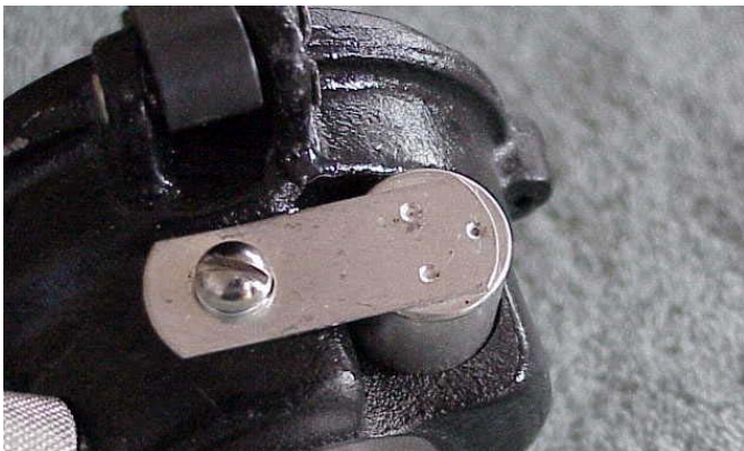
A quality condenser with stake welds
