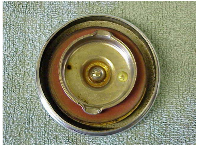
Modified gas cap with a small rivet epoxied into place opposite from the vent hole.
