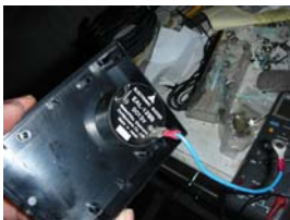
This photo shows the electronic buzzer mounted thru a hole in the box cover.
