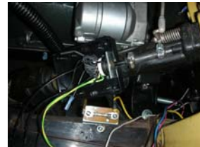
The box fastened to the steering column and the switch connected with the hose. 3" piece of 1/4 id rubber hose and 2 hose clamps
