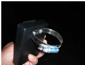
This photo shows the hose clamp mounted to the box
