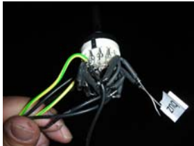
This photo shows the switch with the diodes and wires, and a wiring mistake.
