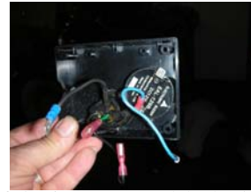
Inside of the box cover with the buzzer and flasher mounted.
