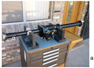
I can also build up a rear end with all new bearings and seals, and with the choice of a good serviceable 378 or 411 ring & pinion and with serviceable axles, and attach the overdrive to it. The proper pre-loads and the backlash will also be set. Or I can rebuild your rear end in the same manner and attach the overdrive.
