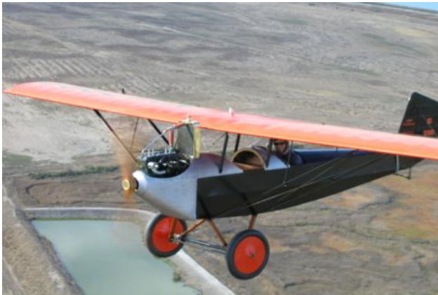
The Model A Powered Pietenpol Air Camper
