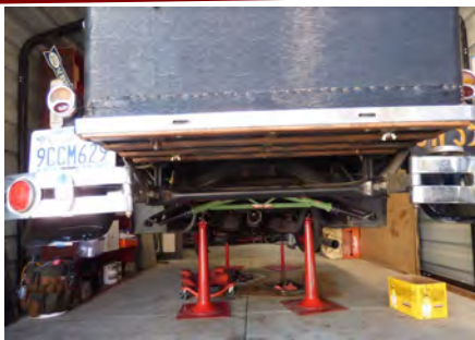
Spring Spreader in place.
