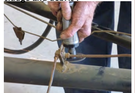
Hyd. Brake lines needed removing.
