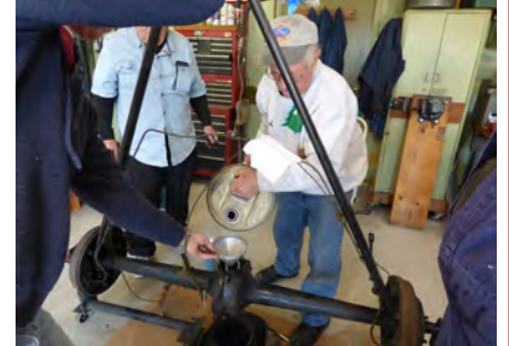
Pouring thinner in to remove sludge and debris.
