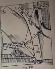
See that there is a slight clearance between fender apron and hood shelf, also between dust shield and hood shelf. That the hood shelf is shield and hood shell. I hat the nood shell is not rubbing against radiator shell or the bumper arm. That there is some clearance between radiator splash shield and front cross member—that the hood clips have not been allowed to become dry or rusted.
